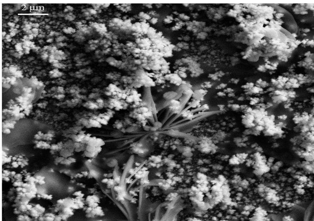
Figure 1. A FESEM image of the electrodeposited gold surface
